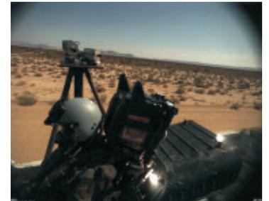
Hi G Seat Ejection Testing
