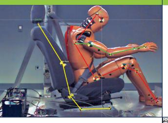
ProAnalyst enables the user to track features without having to use special markers, such as ping-pong balls, in the experimental setup. The Automatic Tracking tools find and track natural features in each video frame.
